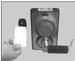
If access control is present – the X09 combination lock bolt must be retracted first and then present the badge and/or PIN. After the access control badge has been accepted, the external lever handle can be turned up or down to retract the deadbolt and open the door.
